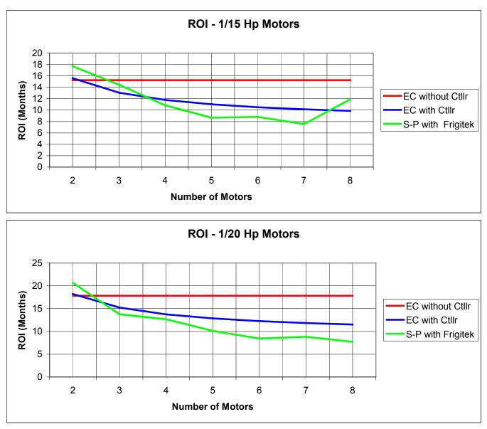
It is interesting to note that EC motors alone provide the longest (and least desirable) ROI time, except for the twomotor scenario. Also, the jump in ROI time seen for the 1/15 Hp transition from seven motors to eight motors is due to the need for a different Classic Frigitek model to handle the higher current of the eight-motor configuration.
