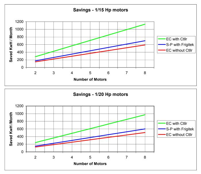
In all cases, the use of the Classic Single-Phase Frigitek with the original shaded-pole motors provides more savings than the EC motors alone.
